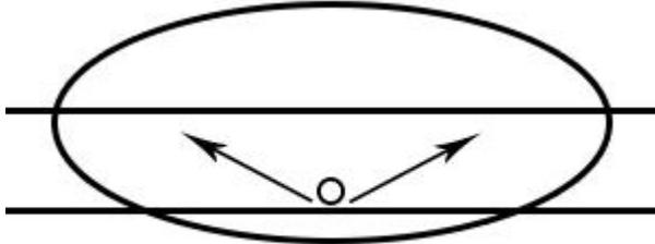
It's best for illuminating the perimeter of parking areas and businesses. The intensity of the Type IV lighting has the same intensity at angles from 90 degrees to 270 degrees.
