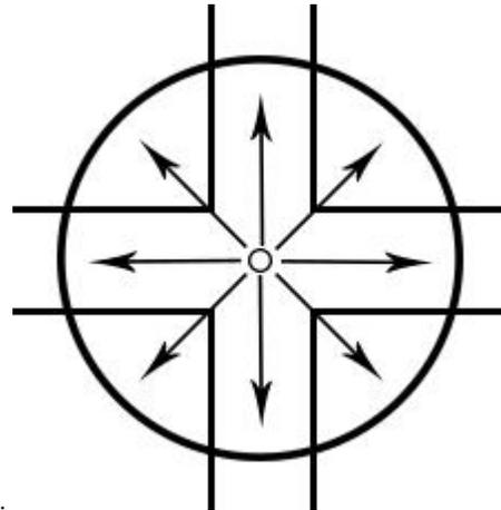
Type V produces a circular distribution that has the same intensity at all angles.
